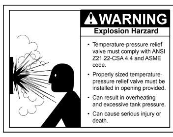
Manually operate the temperature and pressure relief valve at least once a year to make sure it is working
